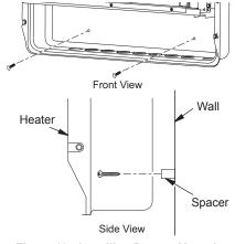
Figure 12 - Installing Bottom Mounting Screws
